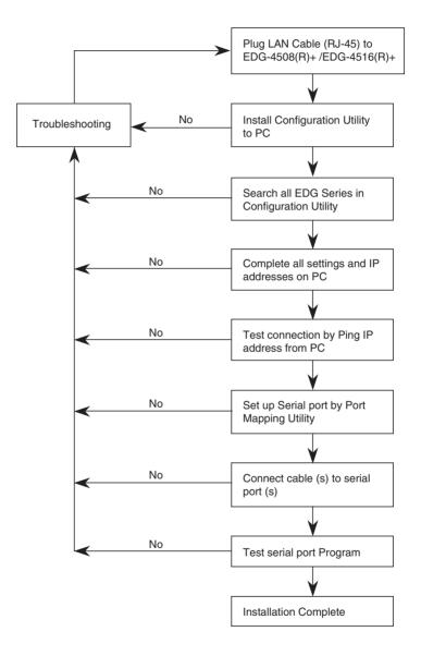
Figure 2.1: Installation Flow Chart
